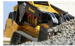
UNIVERSAL ATTACHMENT PLATE. The universal attachment plate provides maximized productivity by giving the operator the ability to change attachments on challenging jobs.
