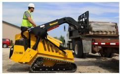
HIGH-CAPACITY LIFTING. The vertical lift capability on the CTX160 boasts a rated (SAE) operating capacity of 1600 lb (725.7 kg) and a hinge pin height of 88.75 in (225.4 cm).
