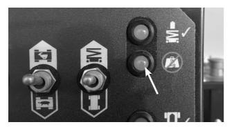
Figure 4.4 – Platform Overload Light
