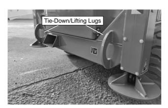
Figure 9.3 – Lifting Lug Points
