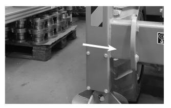
Figure 9.2 – Front Tie-Down/Lifting Lugs
