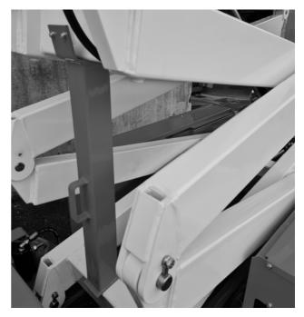
Figure 7.2 – Safety Prop in Support Position
