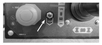
Figure 4.10 – Operator Horn
