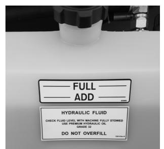
Figure 5.3 Hydraulic Oil Tank
