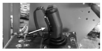
Figure 4.8 – Joystick Interlock Switch
