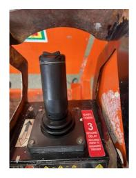
When using the controller hold trigger for 3 seconds before moving
