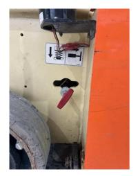
Emergency release to bring the scissor down if it gets stuck in the air.
