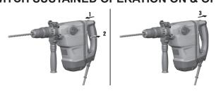
When chiseling, the control switch can be locked in the "on" position.
