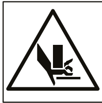
Risk of getting crushed - moving parts
