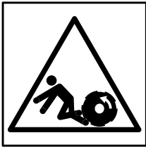
Risk of getting crushed - moving parts
