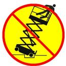
Do not use the platform controls to free a platform that is caught, snagged or otherwise prevented from normal motion by an adjacent structure. All personnel must be removed from the platform before attempting to free the platform using the ground controls.
