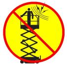
Maintain safe distances from electrical power lines and apparatus in accordance with
