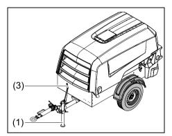
Fixed towbar with support leg and brakes
