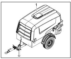
When lifting the compressor, the hoist has to be placed in such a way that the compressor, which must be placed level, is lifted vertically. Keep lifting acceleration and retardation within safe limits.
