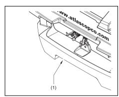
The compressor is fitted with a leak-proof undercarriage in order to protect the environment.
