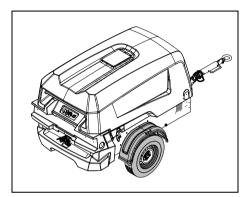
The compressors type XAS 98 Kd, XAS 98G Kd are silenced, single-stage, oil-injected screw compressors, built for a nominal effective working pressure of 7 bar (102 psi) (see chapter **Technical specifications**).
