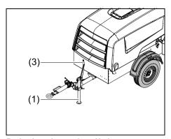
Fixed towbar with support leg and brakes
