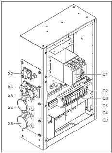
X2 ...... 1-phase outlet socket (230 V AC) Provides phase L3, neutral and earthing.
