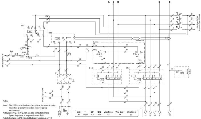
Note 3: Contacts on S10 indicated between brackets, e.g.(T10) aren't to be connected. They are linked internally.
