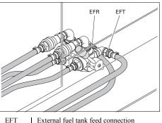
EFI External fuel tank feed connection EFR External fuel tank return connection When using this option, make sure to connect the fuel supply line as well as the fuel return line. Connections to fuel lines ought to be air-tight to prevent air from entering the fuel system. Turn the handle of the valve to desired condition.
