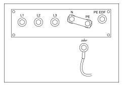
When EDF-option is installed, the unit operates as EDF-unit when the earthing, the PE and the PE EDF terminals are connected to each other (see figure below). In this case, an earth leakage at the side of the generator will switch off the circuit breaker. An earth leakage at the side of the load will not switch off the circuit breaker.
